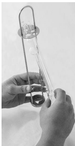
Fig. 5 Inserting or replacing a viscometer with light-barrier sensing
